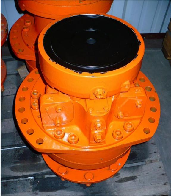
Wheel motor with P35 brake. Note brake cover is held in place with a snap ring.
