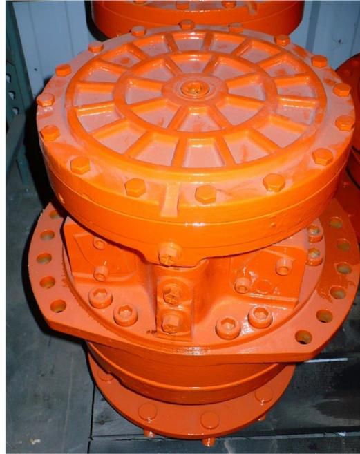
Wheel motor with F35 brake. Note brake cover is held in place with bolts.
